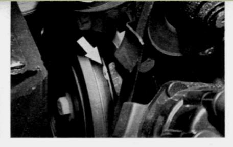
A BURR ON THE timing mark cut into crankshaft pulley has, in some cases, gradually whittled away at Monza fan belts. The factory says warranty records don't show the problem, but owners might do well to check it
