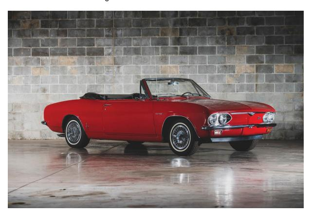
Originally designed to compete with the Volkswagen Beetle, the Corvair actually followed the Bug by ditching its radiator and installing an air-cooled, horizontally-opposed flat-six engine in back. The 1965–69 versions carried a 2.7-liter powerplant that produced 90–140 horsepower, mated to a three-speed or four-speed manual transmission or Powerglide automatic.
