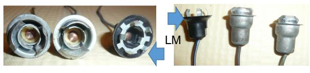
Replace the LM Corsa tack bulb sockets with the EM version
