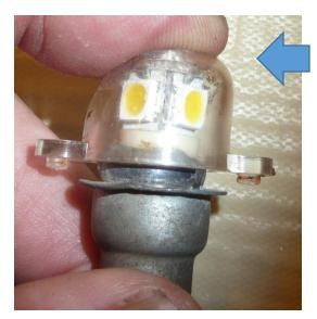
LED is to long and will not fit in Tack with plastic diffuser installed.
