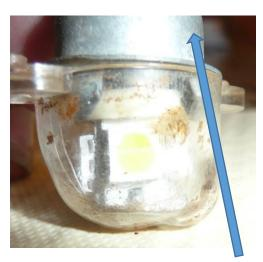
Bulb installed past stop, will fit in tack.
