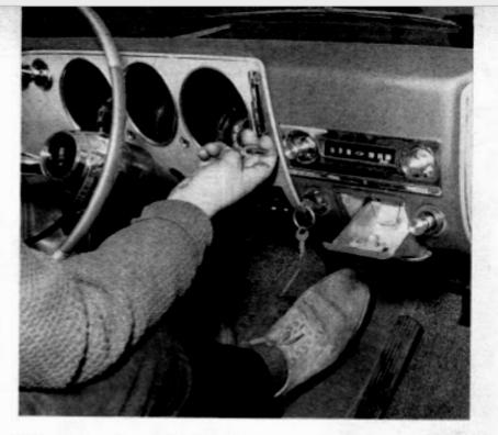
GAUGES ARE DEEPLY recessed, yet readable. Powerglide control is inconvenient, one engineer felt, but other owners didn't find it worthy of comment. PM testers found no distracting windshield reflections at night
